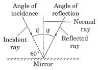
The angle between the plane mirror and the normal ray is 90°. An incident ray strikes the plane mirror at 60° to the normal ray and gets reflected.
