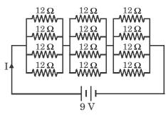
Therefore, the effective resistance of the network of resistors,
