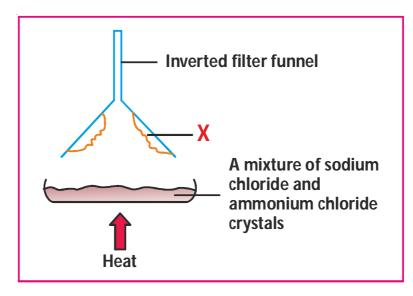
During heating, ammonium chloride crystals turn into vapour. The vapour condenses and crystallises on the cool surface of the inverted filter funnel.
